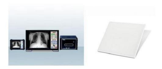
It is based on the cassette-size digital flat panel detector featuring amorphous Silicon (a-Si) technology and a Caesium Iodide (CsI) scintillator, that for its standard formats (35x43 cm and 24x30 cm) can be used inside traditional bucky and cassette-holder of any analogue x-ray rooms.
